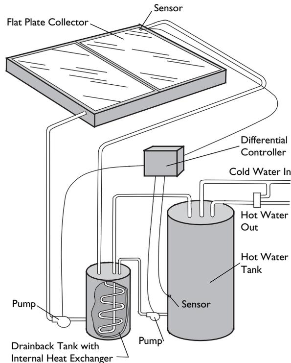
Fig. 6: Drainback solar water heating system.
