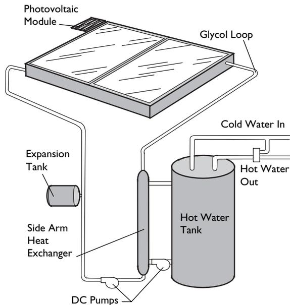
Fig. 7: Pressurized glycol solar water system.
