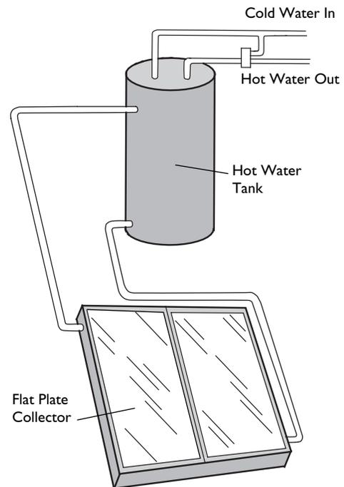
Fig. 8: Thermosiphoning solar water system.
