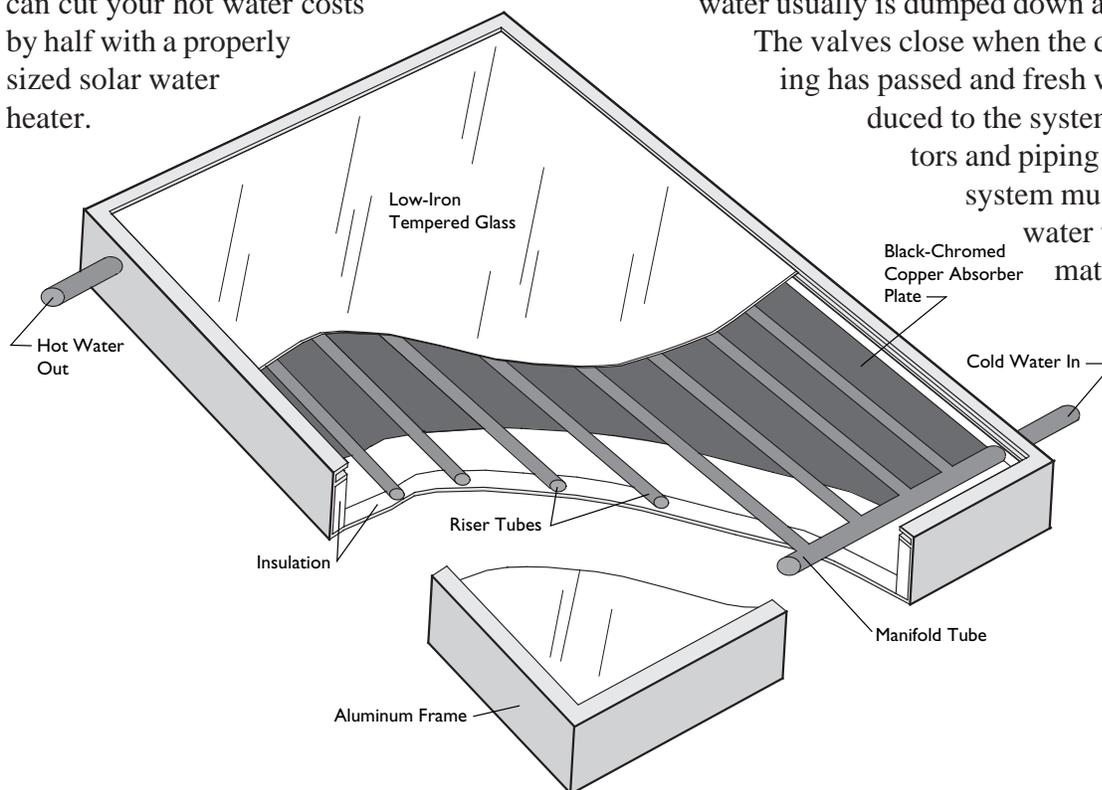
Fig. 4: Cut-away drawing of a typical solar collector.
