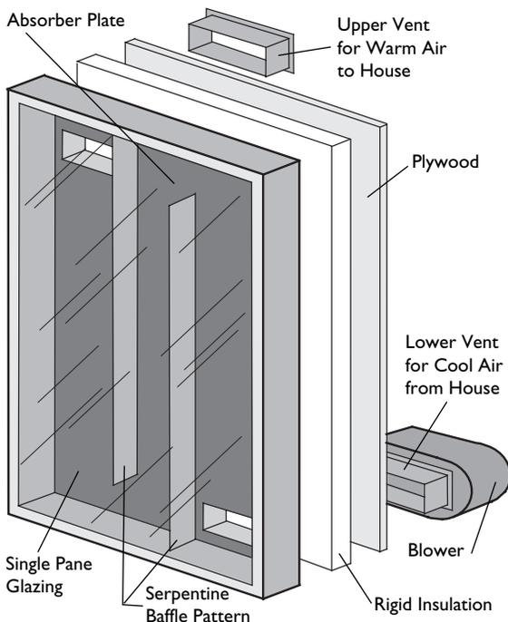
Fig. 21: Active solar wall panel collector.
