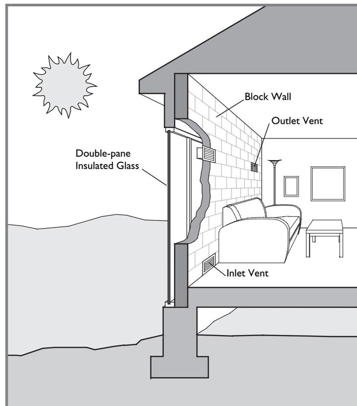
Fig. 14: Indirect passive solar Tromb  wall.
