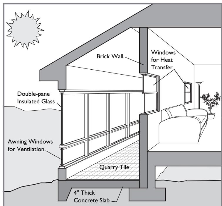
Fig. 15: Isolated passive solar attached greenhouse.
