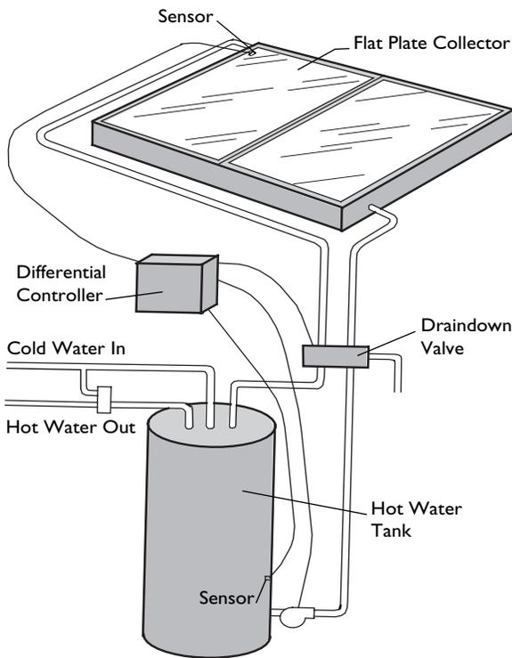
Fig. 5: Draindown solar water heating system.
