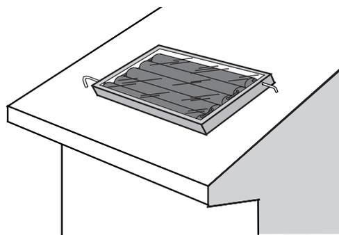
Fig. 10: Integral collector storage system.
