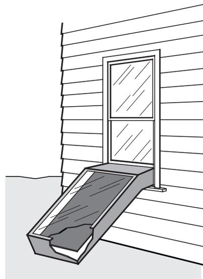
Fig. 20: Window box solar collector.
