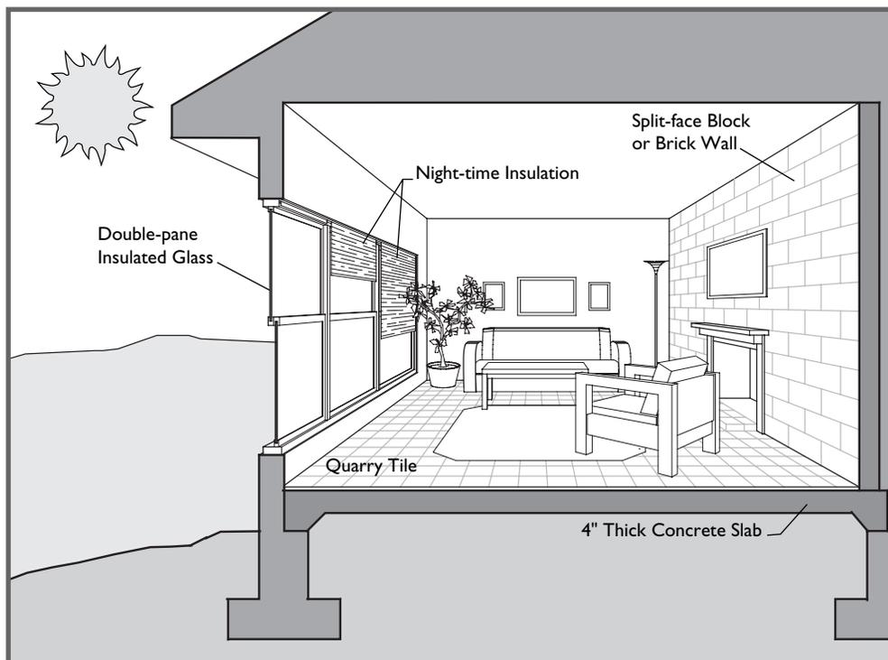
Fig. 13: Cut-away drawing of a direct gain passive solar house.
