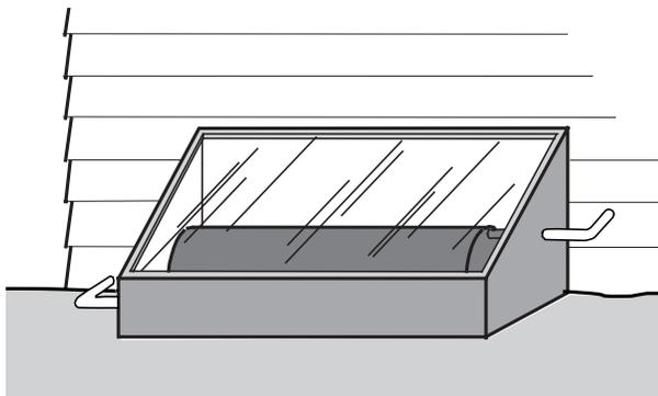
Fig. 9: Breadbox batch solar water heater.
