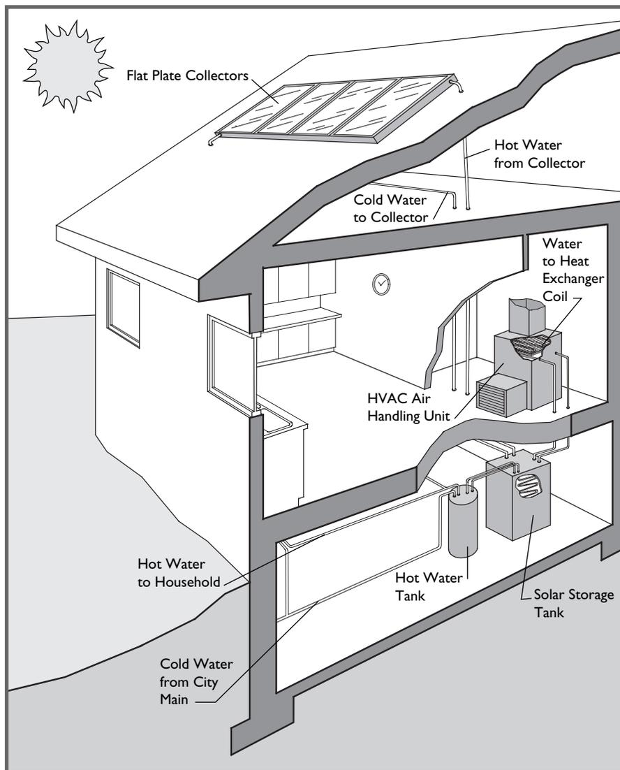
Fig. 2: Cut-away drawing of an active solar heated house.
