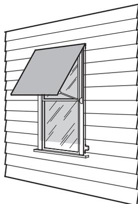
Fig. 18: Retractable awning.
